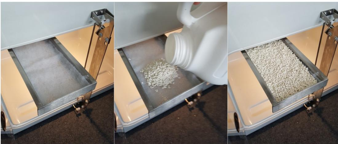
The soda lime drawer should be filled with soda lime up to a height of about 1.5 to 2 cm (approx. 0.7 inches).
